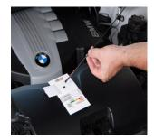
**FLUIDcheckUP** works the same way for all operating fluids: Fluids for all the above-mentioned systems contain important additives, designed to prevent damage and protect the oils from overheating, wear, aging. When these additives are aged or used up, oil sludge forms. Also, water and abrasion in the operating oils can affect their functional capabilities.
